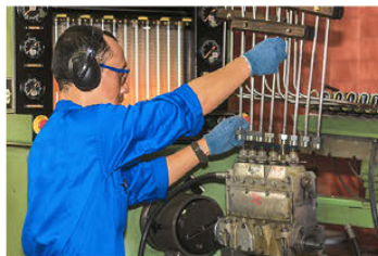
Calibration Injection Pump in Line
